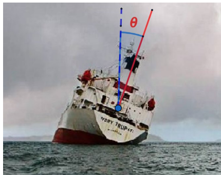
Figure 8.3 Rolling of a vessel
